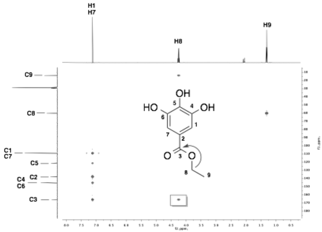
Figure 3.7 ^1\text{H} - ^{13}\text{C} gHMBC of ethyl gallate acquired using 4 scans and 200 increments and optimized to 8Hz.
